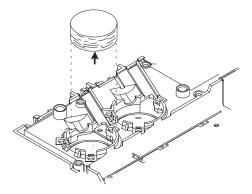
4. Carefully remove the scribed circle of insulation from the front or back inlet position to create an opening into the oven, if necessary.
