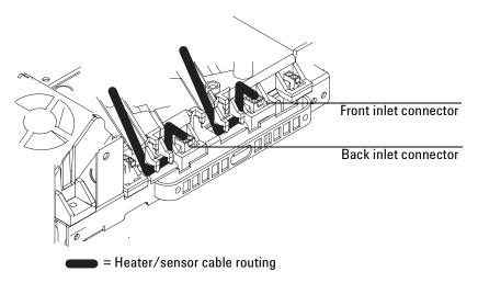
5. Place the trap in in the compartment at the end of the pneumatics carrier. Route the trap's copper tubing behind the fan bracket and to the inlet. Route the trap's stainless steel tubing behind the fan and to the flow manifold. Route the stainless steel tubing from the inlet to the flow manifold.
