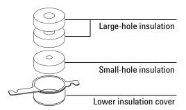
6. From inside the oven, install the two heat-resistant screws in the cutouts adjacent to the inlet opening. Do not tighten the screws. Push the lower insulation cover over the front or back inlet until it is flush with the oven top and rotate it until the slots in the cup hook over the screws. Tighten the screws with a Torx T-20 screwdriver.
