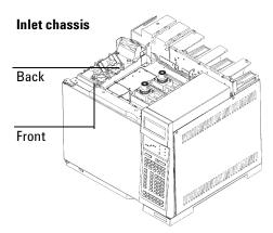
2. Remove the round metal cutout in the front or back inlet position, if necessary. Insert a flat-blade screwdriver into the slot in the cutout and move the screwdriver back and forth until the cutout breaks free from the sheet metal on the oven top.
